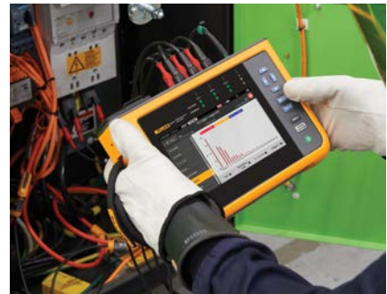
Captures all the key measurements you need to determine power quality health.
